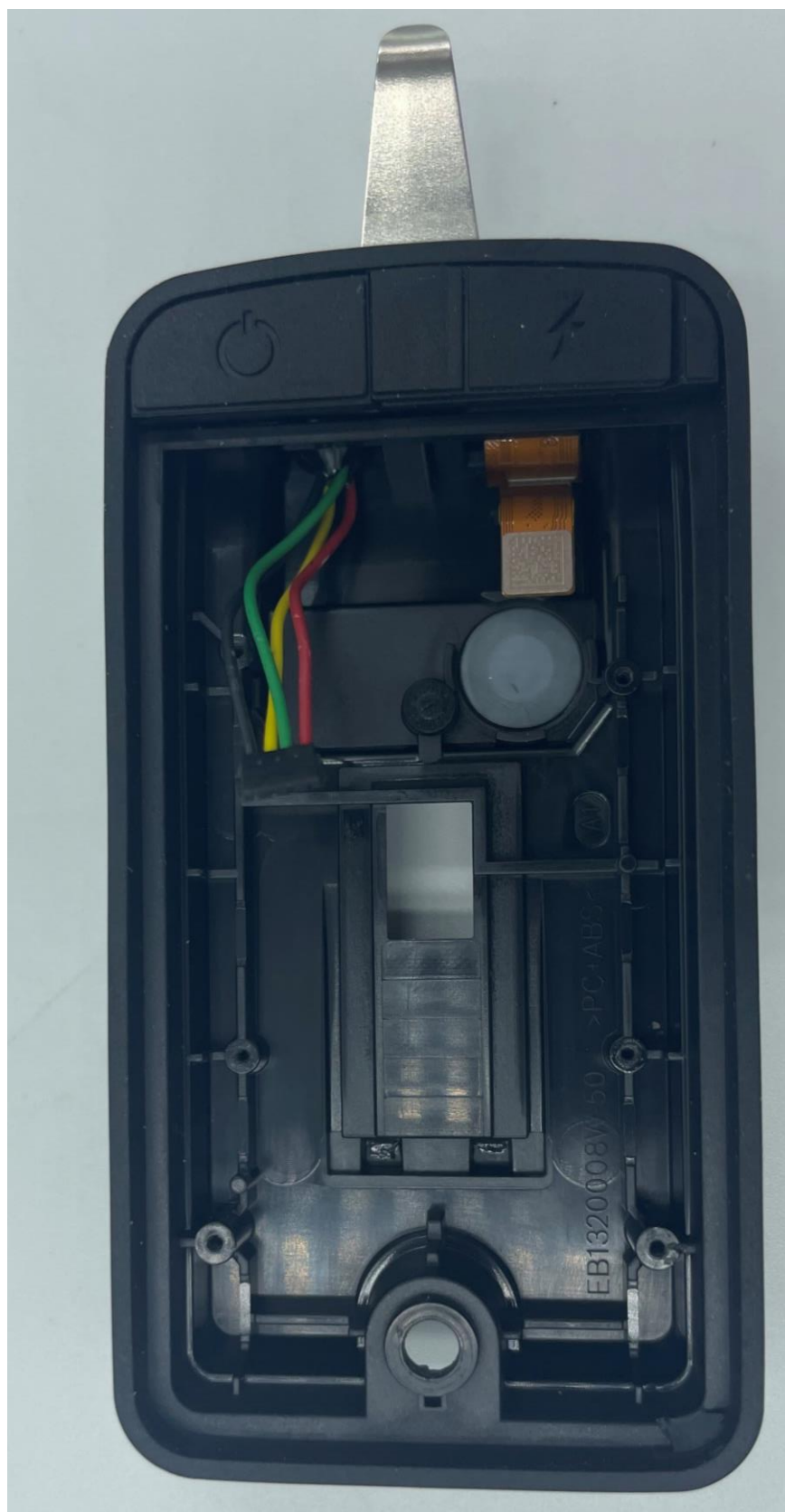
Figure 12: BRC3200 bottom housing w/o battery
